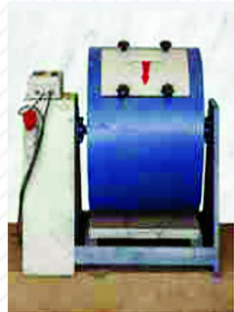
LOS ANGELES ABRASION TESTING MACHINE
